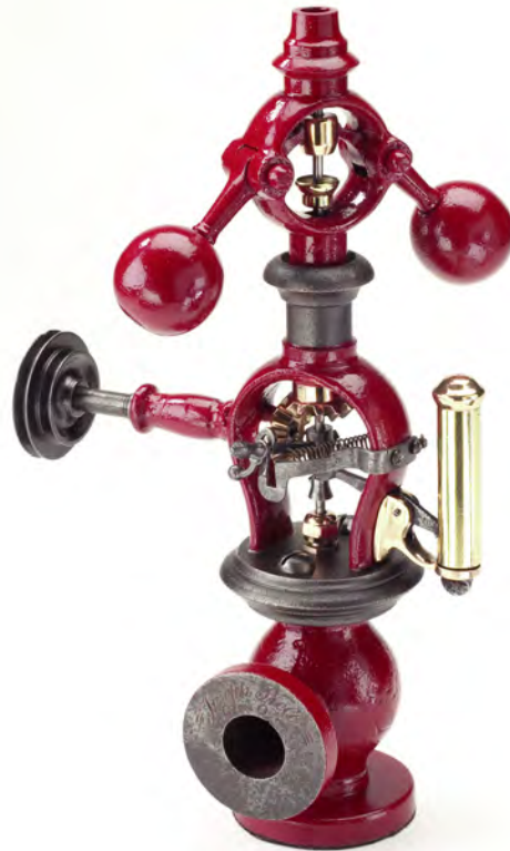
Governor for Steam Engines, 1870. Joseph Bell, Cincinnati, OH.
