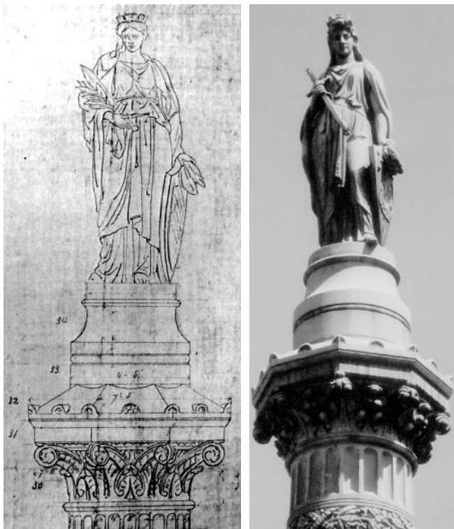
L to R: Drawing of the top of the Buffalo monument, as published in the 20 th Annual Report Buffalo Park Commission, 1890, showing the pieces numbered to assist in assembly. The top of the monument, as seen today. Photograph by author.
